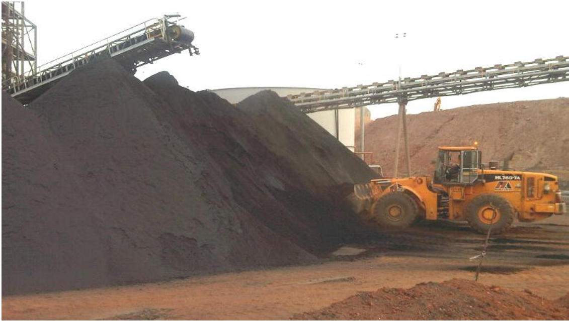
Magnetite concentrate from the CMB plant ready for roasting in the rotary kiln
