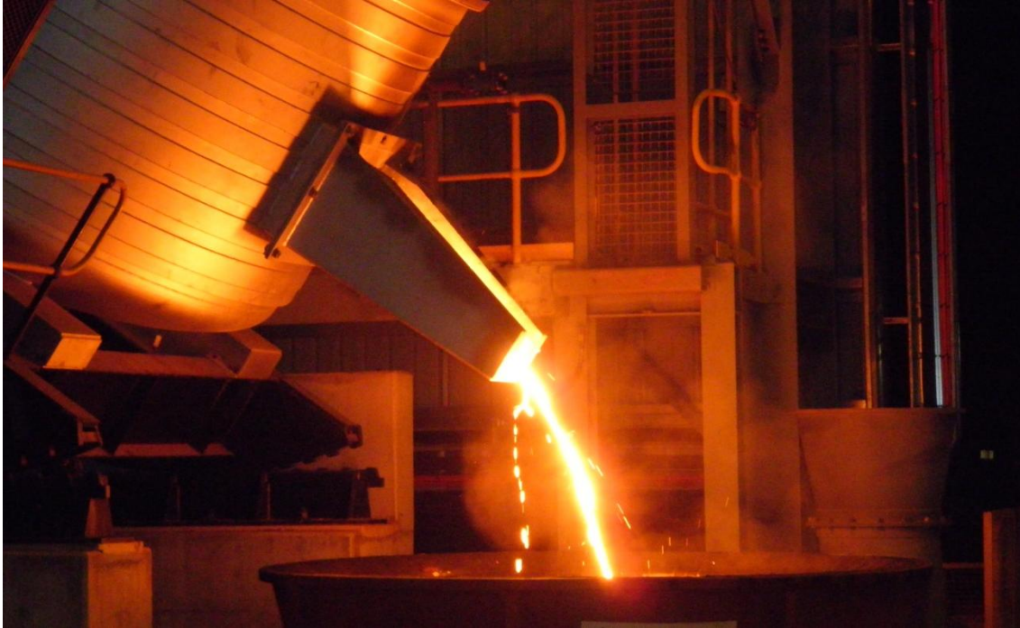
Ferrovandium electric arc furnace undergoing commissioning with a slag and steel mix
